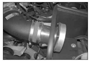
28. Install the mass air sensor assembly onto the intake tube, then secure with the provided hose clamp.
