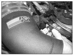
24. Install the temp sensor into the intake tube then reconnect the electrical connection as shown.
