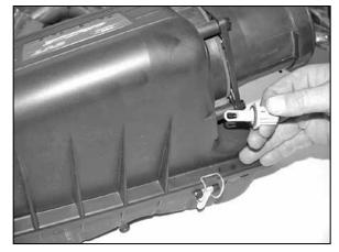
23. Remove the temp sensor from the factory air box as shown.
