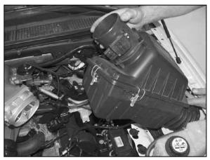
6. Pull up firmly on the factory air box to remove from vehicle.
