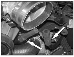
20. Install the two provide 5/8 silicone hoses onto the idle air and crank case vent lines as shown.
