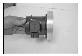
26. Assemble the filter adapter and gaskets onto the mass air sensor with the provided hardware as shown.
