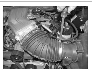
3. Loosen the hose clamp at the throttle body and
