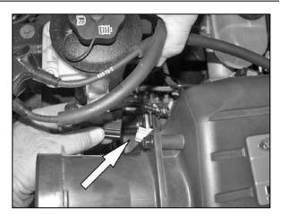
5. Disconnect the temp sensor electrical connection
